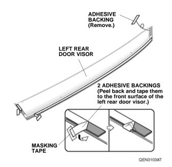
16. Remove the adhesive backing.
