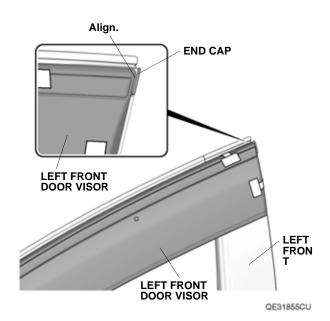
9. While applying light pressure against the left front door visor, carefully remove the adhesive backings in the order shown. Make sure to push up on the brackets while removing the adhesive backings.
