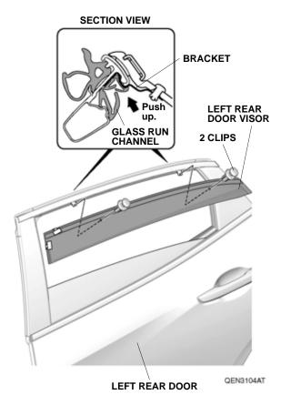
Secure the left rear door visor to the two brackets with the two clips. Make sure to push up on the brackets while installing the two clips.
