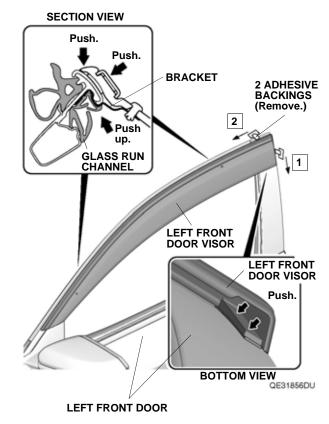
10. Using a soft towel, press and hold the left front door visor against the door sash for 30 seconds.
