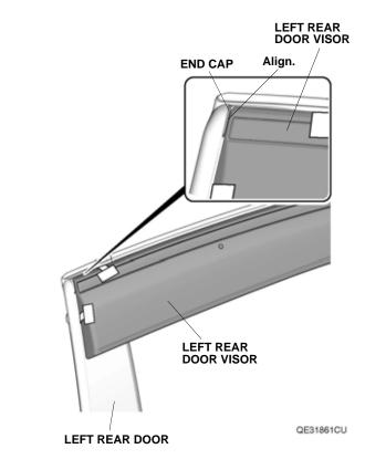
20. While applying light pressure against the left rear door visor, carefully remove the taped adhesive backings in the order shown. Make sure to push up on the brackets while removing the adhesive backings.
