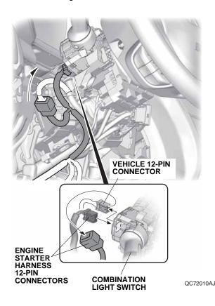
59. Align the white tape on the engine starter harness with the vehicle clip, and secure the engine starter harness and engine starter harness 12-pin connector to the vehicle harness with one wire tie.
