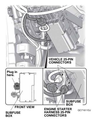
51. Secure the engine starter harness 25-pin connector and engine starter harness to the vehicle harness with one wire tie and one long wire tie.
