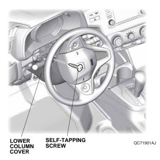
17. Turn the steering wheel 180° clockwise, and remove the self-tapping screw from the lower column cover.
