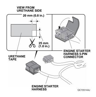
63. Unplug the vehicle 5-pin connector, and plug it into the engine starter harness 5-pin connector. Plug the remaining engine starter harness 5-pin connector into the vehicle 5-pin connector.
