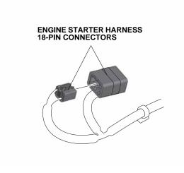
29. Attach the engine starter harness clip onto the vehicle 18-pin connector.
