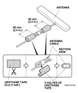
20. Using scissors, cut three urethane tapes in half. Starting near the antenna end of the cable, wrap five halves of urethane tape around the antenna cable at the measurements shown.
