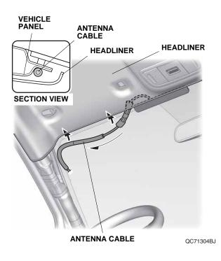
23. Route the antenna cable along the A-pillar as shown. Secure the antenna cable to the vehicle harness with four wire ties.
