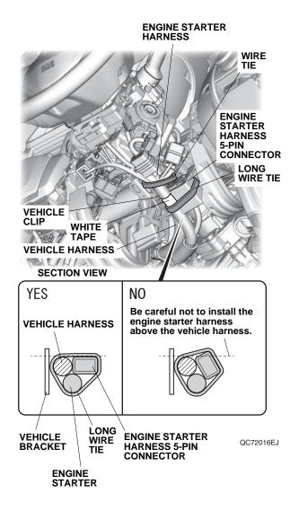
65. Secure the engine starter harness and antenna cable to the knee bolster with one long wire tie.
