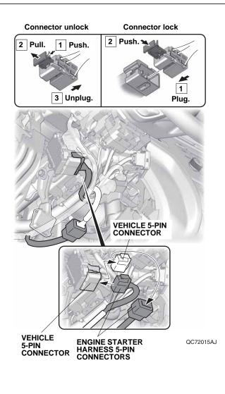
64. Align the white tape on the engine starter harness with the vehicle clip, and secure the engine starter harness and engine starter harness 5-pin connector to the vehicle harness with one wire tie and one long wire tie.
