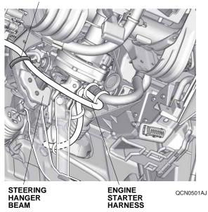
55. Route the engine starter harness along the vehicle harness. Align the white tape on the engine starter harness with end of the vehicle harness protector, and secure the engine starter harness to the vehicle harness with one wire tie.
