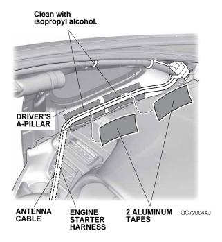
33. Attach the antenna cable and engine starter harness to the driver's A-pillar with two aluminum tapes.
