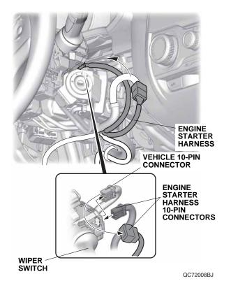
57. Align the white tape on the engine starter harness with the vehicle clip, and secure the engine starter harness and engine starter harness 10-pin connector into the vehicle harness with one wire tie.
