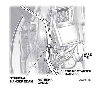
35. Secure the antenna cable and engine starter harness to the vehicle harness with one long wire tie.
