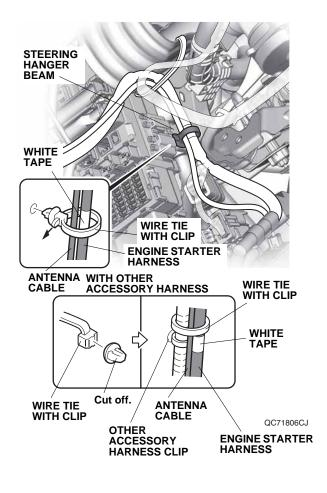
67. Bundle up the excess antenna cable as shown, and wrap one urethane tape around the antenna cable. Secure the antenna cable to the engine starter harness with one wire tie.
