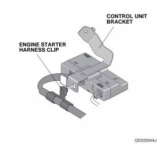
45. Secure the subfuse box bracket (removed in step 39) and control unit bracket to the studs with two nuts as shown.
