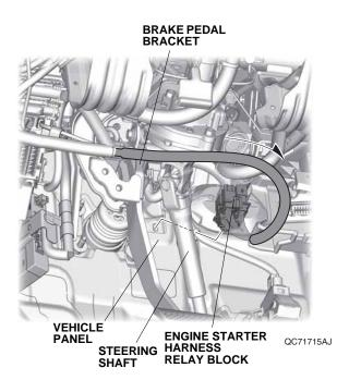
53. Align the white tape on the engine starter harness with the vehicle clip, and secure the engine starter harness to the vehicle harness with four wire ties.
