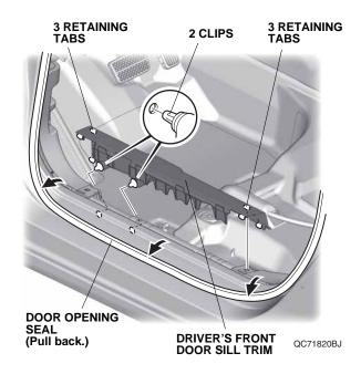
11. Pull back the door opening seal, and remove the driver's kick panel.
