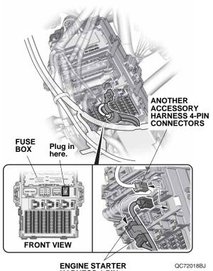
HARNESS 4-PIN CONNECTORS 50. Unplug the vehicle 25-pin connector, and plug it into the engine starter harness 25-pin connector. Plug the remaining engine starter harness 25-pin connector into the vehicle 25-pin connector.
