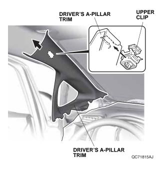
6. Remove the remaining upper clip from the driver's A-pillar.
