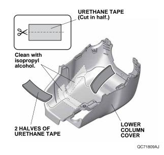
71. Using scissors, cut one urethane tape in half. Attach two halves of urethane tape to the lower column cover as shown.
