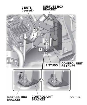
46. Install the subfuse box released in step 38.
