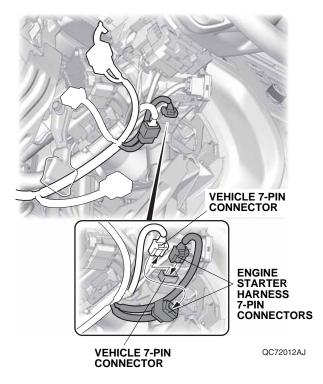
61. Secure the engine starter harness 7-pin connector into the vehicle harness with one wire tie.
