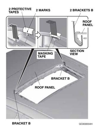
10. Place the two brackets A into position over the two protective tapes and around the lip of the roof panel, and tape them into position with masking tape. Be sure to align the lower end of the brackets A with the second indentation.
