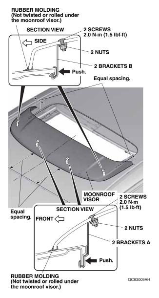
Tighten while applying pressure so that there is no gap between the roof panel and the brackets A and B. Torque the screws to 2.0 N·m (1.5 lb·ft). 15. Remove the shop towels inserted in step 2. Remove the IMPORTANT INFORMATION label.
