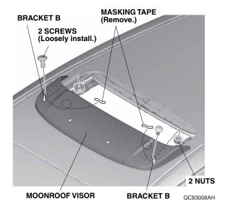
Position the moonroof visor with equal spacing in the front and on the sides. Check that the rubber molding is not twisted or rolled under the moonroof visor.
