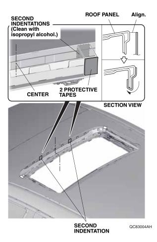
8. Remove the adhesive backings from two of the protective tapes, and attach them to the roof panel at second indentation.
