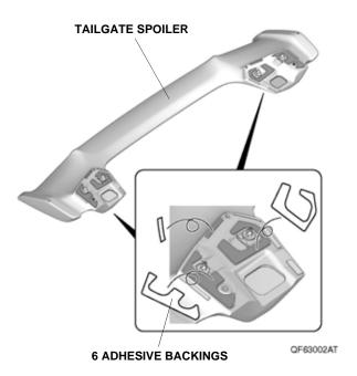
10. With the help of an assistant, position the tailgate spoiler on the tailgate and loosely install the two bolts.
