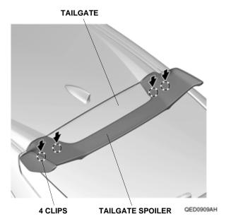
12. Hold the tailgate spoiler firmly against the tailgate over the adhesive tapes with the palm of your hand for 30 seconds.
