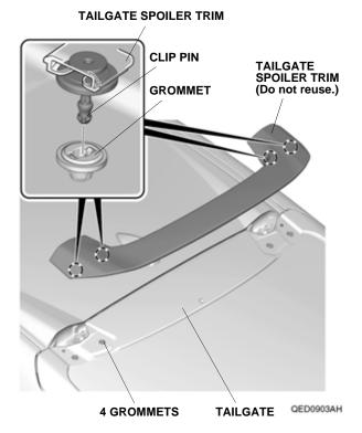
3. Remove the four grommets from the tailgate.
