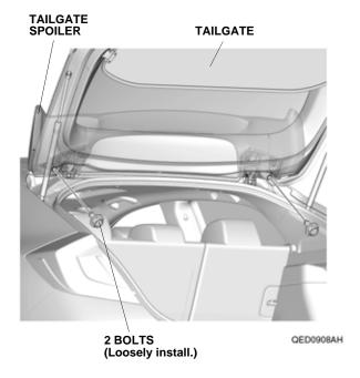
11. Apply pressure to the tailgate spoiler over each clip until you hear a click. Do not apply excessive pressure.
