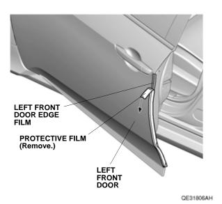
12. Starting from the center and working outward, use your fingers to fold the left front door edge film around the edge of the left front door as shown. Move your fingers in one direction only. Attach the left front door edge film over the seam sealant. Do not trim or damage the seam sealant.
