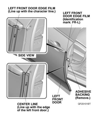
4. Line up the center line on the left front door edge film with the edge of the left front door. While applying light pressure, carefully remove the adhesive backing, and attach the left front door edge film to the left front door. Go to step 10.
