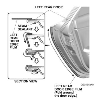
23. Using a shop towel, wipe the excess 3M protective tape application solution from the left rear door edge film. Allow the left rear door edge film to dry thoroughly.
