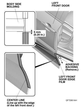
9. Line up the center line on the lower part of left front door edge film with the edge of the left front door. While applying light pressure, carefully remove the adhesive backing and attach the lower part of the left front door edge film to the left front door. 10. Insert the applicator into the soft sleeve. Starting from the top and working downward, use the soft sleeve to smooth the left front door edge film. Move the soft sleeve in one direction only.
