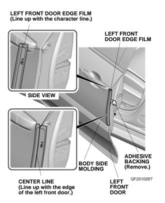
7. Line up the center line on the upper part of left front door edge film with the edge of the left front door. While applying light pressure, carefully remove the adhesive backing and attach the upper part of left front door edge film to the left front door. 8. Peel back about 50 mm (1.97 in.) of adhesive backing from the lower part of left front door edge film. Line it up as shown.
