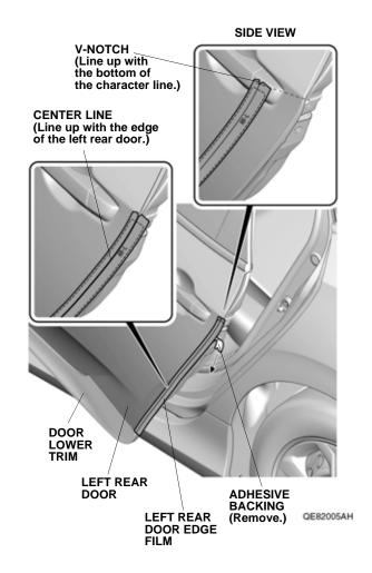
19. Line up the center line on the left rear door edge film with the edge of the left rear door. While applying light pressure, carefully remove the adhesive backing and attach the left rear door edge film to the left rear door. 20. Starting from the top and working downward, use the soft sleeve to smooth the left rear door edge film. Move the soft sleeve in one direction only.
