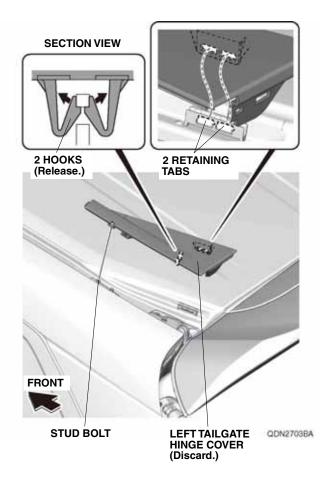
4. Remove and discard the two clips from the two stud bolts on the roof.
