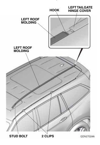
Open the tailgate. Using a plastic trim tool, release the left tailgate hinge cover extension.
