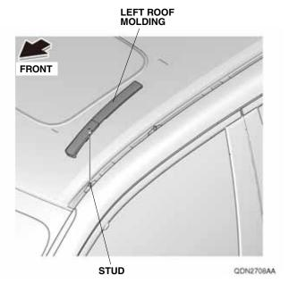
Install the left roof rail base to the three stud bolts with three 6 mm TORX nuts. Make sure the roof rail base is installed in the correct position. Torque the 6 mm TORX nuts to 6.9 - 11.8 N·m (5.1 - 9 lbf·ft).
