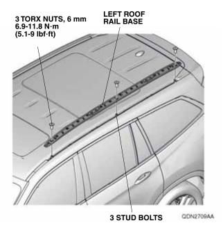
Secure the left roof rail base to the four stud bolts with four 8 mm TORX nuts.
