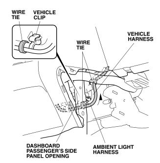
15. Route the ambient light harness along the vehicle harness, and to the blower motor. Secure the ambient light harness to the vehicle harness with two wire ties. Secure the wire tie next to the vehicle clip.
