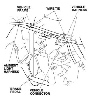
13. Route the ambient light harness through the center console, and secure it to the vehicle harness with three wire ties. Secure the wire tie next to the vehicle clip.
