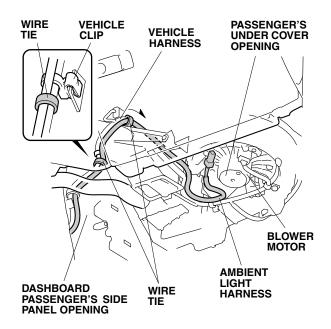
16. Secure the ambient light harness to the vehicle harness with three wire ties. Secure the wire tie next to the vehicle clip.
