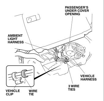
17. Install the ambient light into the passenger's under cover as shown.
