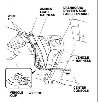
14. Route the ambient light harness along the vehicle harness, and secure it to the vehicle harness with two wire ties. Secure the wire tie next to the vehicle clip.
