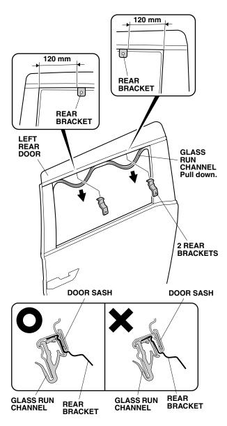
13. Reinstall the glass run channel to secure the two rear brackets. Be sure the brackets are installed tightly to the door sash, and that the glass run channel is properly seated.  Using isopropyl alcohol on a shop towel, thoroughly clean the door where the left rear door visor will attach.
