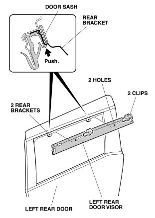
17. Secure the left rear door visor to the front brackets with two clips. Push up on the rear brackets while installing the two clips. Install the clips correctly, they cannot be removed.
