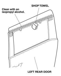
15. Peel back 1½ to 2 inches of each adhesive backing, and tape the ends to the front surface of the left rear door visor with masking tape.
