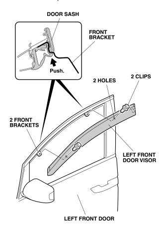
7. Secure the left front door visor to the front brackets with two clips. Push up on the front brackets while installing the two clips. Install the clips correctly, they cannot be removed.
