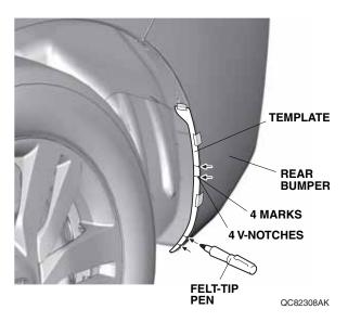
14. Carefully remove template. Do not damage the template, it will be also used to mark the right rear bumper.
