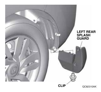
17. Secure the left rear splash guard the two 5 x 20 mm self-tapping screws in the order shown below. NOTE: Make sure there is no gap between the left rear splash guard and the bumper. If there is a gap, loosen the self-tapping screws, press and hold the splash guard against the bumper with the palm of your hand, and tighten the screws.
