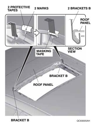
10. Place the two brackets A into position over the two protective tapes and around the lip of the roof panel, and tape them into position with masking tape. Be sure to align the lower end of the brackets A with the second indentation.
