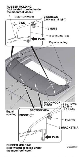
Tighten while applying pressure so that there is no gap between the roof panel and the brackets A and B. Torque the screws to 2.0 N·m (1.5 lbf·ft). 15. Remove the shop towels inserted in step 2. Remove the IMPORTANT INFORMATION label.
