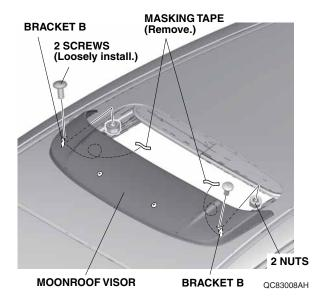
13. Position the moonroof visor with equal spacing in the front and on the sides. Check that the rubber molding is not twisted or rolled under the moonroof visor.
