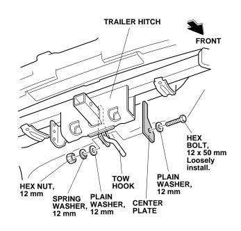
32. Tighten the bolts to the specified torque in the order of  $\boxed{1}$  and  $\boxed{2}$ . Torque the 10 x 40 mm hex bolts to 46 N·m (34 lbf·ft). Torque the 12 x 50 mm hex bolt to 79 N·m (58 lbf·ft).
