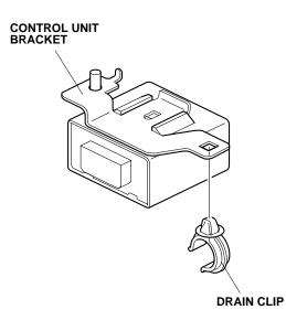
51. Install the control unit bracket to the vehicle panel with one 6 mm flange nut.
