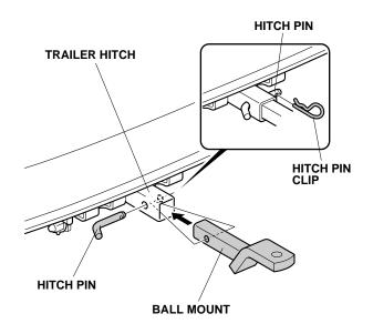
75. Secure the ball mount to the trailer hitch with the hitch pin and hitch pin clip.
