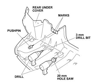
36. While wearing eye protection, drill each pierced mark on the rear under cover. First drill with a 3 mm drill bit, then enlarge each hole to 20 mm using a 20 mm hole saw.
