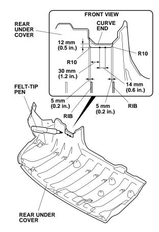
35. Using a pushpin, pierce the center of each mark made in step 34 on the rear under cover.
