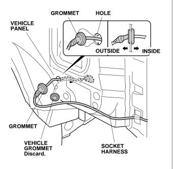
47. Using isopropyl alcohol on a shop towel, thoroughly clean the area where the aluminium tape will attach. Secure the socket harness to the vehicle panel with one additional aluminum tape.
