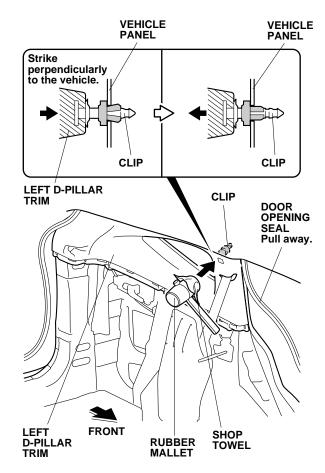
20. Using a rubber mallet wrapped with a shop towel, lightly tap the area marked "SIDE CURTAIN AIRBAG" on the left D-pillar trim to push in the clip. Make sure to strike area perpendicularly to the vehicle. 21. Remove the left D-pillar trim.
