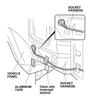
Inside the vehicle, secure the socket harness.
