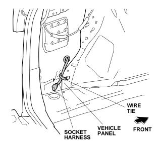
4WD vehicle: Route the socket harness along the vehicle harness and secure it to the vehicle harness with one wire tie.
