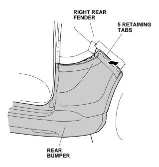
• On each side, release four retaining tabs.
