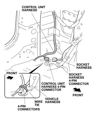
67. Install the connector clip to the fuse case on the control unit harness.
