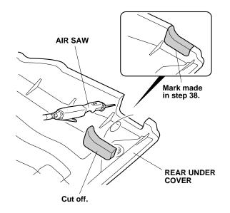
40. Using an air saw, cut the rear under cover along the scribe line as shown. Remove any burrs and sharp edges from the corners.
