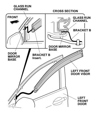
7. Align the clip holes in the left front door visor with the bracket holes, and install the clips while pushing up on each bracket A. There should be no clearance between the brackets and the door sash.
