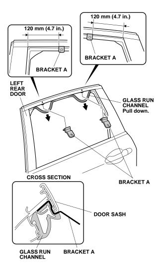
13. Install two brackets A between the door sash and the glass run channel at the measurements shown. Seat the glass run channel properly around the brackets.
