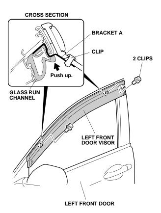
8. Adjust the end gap of the left front door visor as shown.
