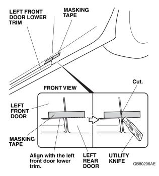
9. Using an utility knife, cut the masking tape along the gap of the left doors. Be careful not to damage the doors.
