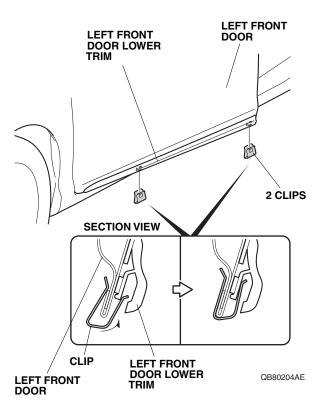
6. Close the left front door. Using a rubber roller, apply firm pressure against the left front door lower trim and roll from one end to the other. Apply firm pressure especially at the ends.
