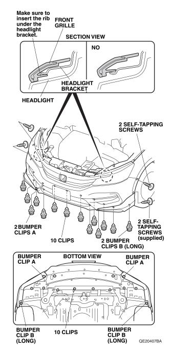
14. Secure the left and right front under spoilers to the front bumper with two bumper clips A, two bumper clips B (long), and two self-tapping screws.
