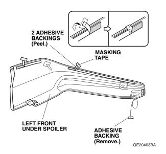
8. Using one alcohol swab, thoroughly clean the front bumper where the left front under spoiler will attach.
