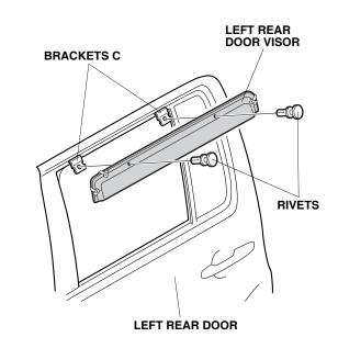
13. Using isopropyl alcohol on a shop towel, clean the door sash where the left rear door visor will attach.
