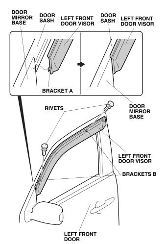
6. Align the holes in the brackets B with the holes in the left front door visor and secure it with two rivets.
