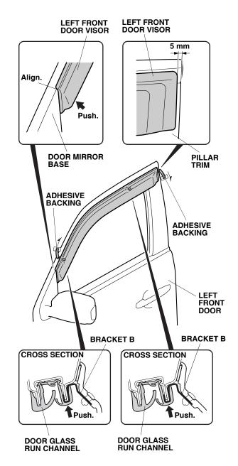
8. Remove the adhesive backings from the left front door visor.
