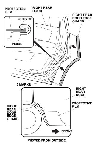
15. Make sure it is positioned correctly, then tap the right rear door edge guard into position with a series of light taps using a rubber mallet. Once in place, do not remove, reposition, or reinstall the right rear door edge guard or it will not hold securely.
