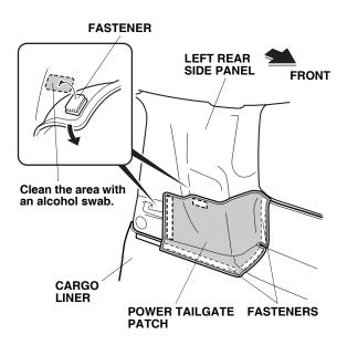
23. Align the power tailgate patch to the left rear side panel. Fold the power tailgate patch back and, using an alcohol swab, thoroughly clean the area where the fasteners will attach. After cleaning with the alcohol swabs, wait at least 3 minutes before continuing with the next step. 24. Attach two fastener pads to the power tailgate patch as shown.
