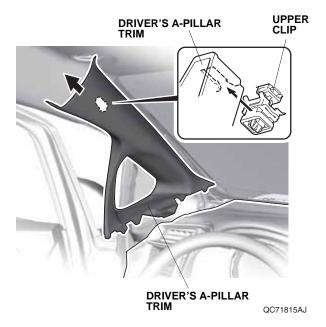
6. Remove the remaining upper clip from the driver's Apillar.
