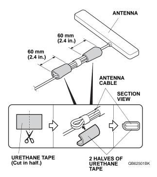
Using scissors, cut three urethane tapes in half.
