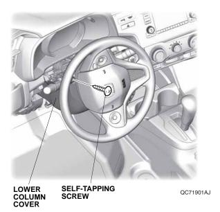
17. Turn the steering wheel 180° clockwise, and remove the self-tapping screw from the lower column cover.
