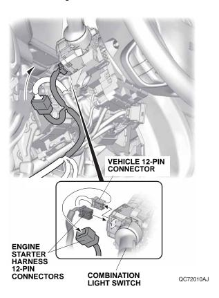
59. Align the white tape on the engine starter harness with the vehicle clip, and secure the engine starter harness and engine starter harness 12-pin connector to the vehicle harness with one wire tie.
