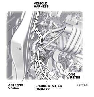
36. Route the engine starter harness along the vehicle harness. Remove the bolt, and install the engine starter harness ground terminal with one ground bolt.
