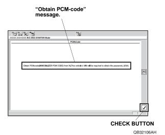
9. Input the PCM-code, then click the check button. NOTE: To ensure security, the PCM-code (password) is changed everyday, so it is impossible to register the remote control engine starter if the dates of the PCM-code acquisition and registration are different. The date of the HDS/MVCI tester should also be the same.
