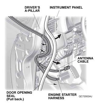
32. Using isopropyl alcohol on a shop towel, clean the driver's A-pillar where the aluminum tapes will attach.
