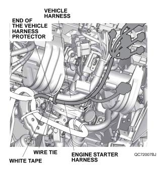
56. Unplug the vehicle 10-pin connector from the wiper switch, and plug it into the engine starter harness 10-pin connector. Plug the remaining engine starter harness 10-pin connector into the wiper switch.
