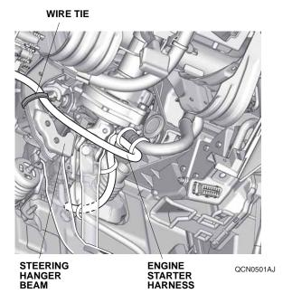
55. Route the engine starter harness along the vehicle harness. Align the white tape on the engine starter harness with end of the vehicle harness protector, and secure the engine starter harness to the vehicle harness with one wire tie.
