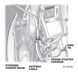
35. Secure the antenna cable and engine starter harness to the vehicle harness with one long wire tie.
