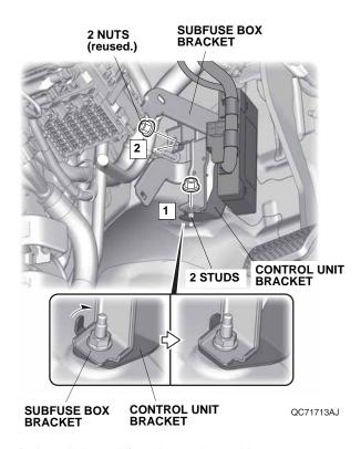
46. Reinstall the subfuse box released in step 38.
