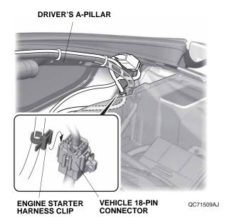
30. Secure the antenna cable, engine starter harness, and engine starter harness 18-pin connector to the vehicle harness with one wire tie.
