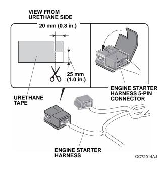
63. Unplug the vehicle 5-pin connector, and plug it into the engine starter harness 5-pin connector. Plug the remaining engine starter harness 5-pin connector into the vehicle 5-pin connector.
