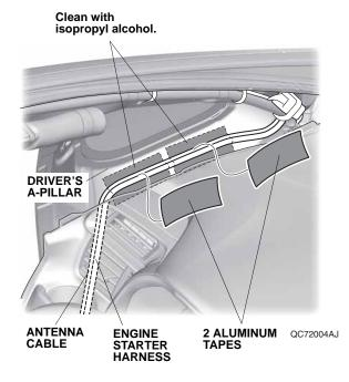
33. Attach the antenna cable and engine starter harness to the driver's A-pillar with aluminum tape.
