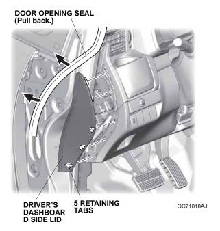
9. Remove the driver's dashboard lower cover, and unplug the vehicle connectors.
