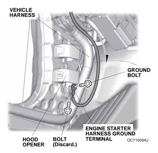
37. Secure the engine starter harness to the vehicle harness with two wire ties.
