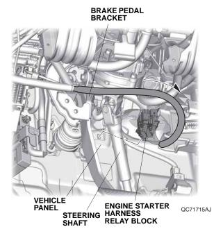
53. Align the white tape on the engine starter harness with the vehicle clip, and secure the engine starter harness to the vehicle harness with four wire ties.
