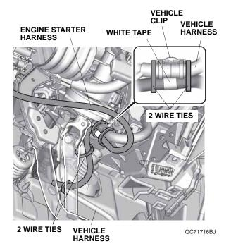
54. Secure the engine starter harness to the steering hanger beam with one wire tie.
