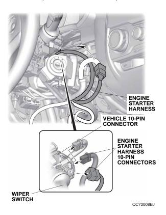
57. Align the white tape on the engine starter harness with the vehicle clip, and secure the engine starter harness and engine starter harness 10-pin connector to the vehicle harness with one wire tie.
