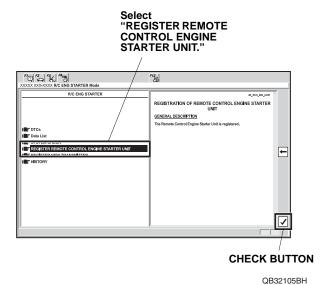
8. The following message will display: Obtain PCM-code (IMMOBILIZER PCM CODE) from iN. This vehicle's VIN will be required to obtain the password. (USA) Click the check button.
