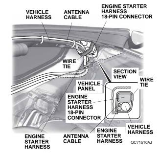
31. Pull back the door opening seal. Route the antenna cable and engine starter harness along the instrument panel, and tuck the antenna cable and engine starter harness between the driver's A-pillar and the instrument panel.
