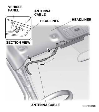
23. Route the antenna cable down the A-pillar as shown. Secure the antenna cable to the vehicle harness with four wire ties.
