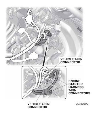
61. Secure the engine starter harness 7-pin connector to the vehicle harness with one wire tie.
