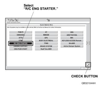
7. Select **REGISTER REMOTE CONTROL ENGINE STARTER UNIT**, then click the check button.
