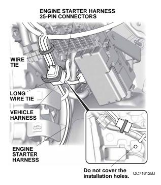
52. Route the engine starter harness behind steering shaft as shown. Secure the engine starter harness relay block to the hole in the vehicle panel.
