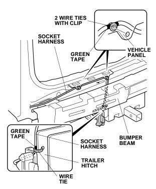
43. At the first green tape, secure the socket harness to the trailer hitch with one wire tie. At the next two green tapes, secure the socket harness to the vehicle panel with two wire ties with clip.
