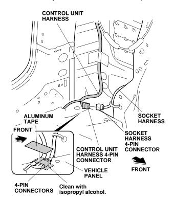
4WD vehicle: Plug the control unit harness 4-pin connector to the socket harness 4-pin connector and secure the 4-pin connectors to the vehicle harness with one wire tie.
