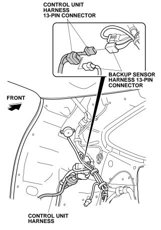
59. Plug the vehicle 13-pin connector into the control unit harness 13-pin connector. Go to step 61.
