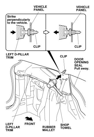
20. Using a rubber mallet wrapped with a shop towel, lightly tap the area marked "SIDE CURTAIN AIRBAG" on the left D-pillar trim to push in the clip. Make sure to strike area perpendicularly to the vehicle.
