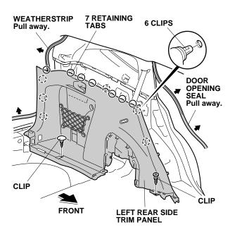
18. Release the wire and remove the left rear seat release lever, then remove the left rear side trim panel.
