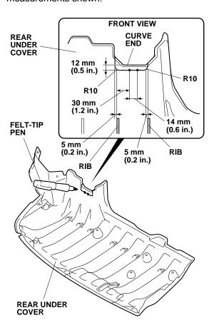
35. Using a pushpin, pierce the center of each mark made in step 34 on the rear under cover.
