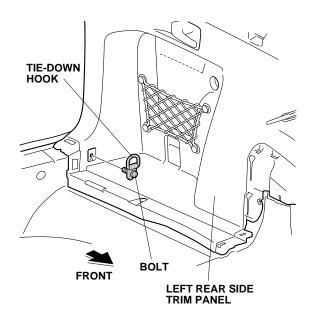
17. Pull away the weatherstrip from around the left rear side trim panel at the tailgate, and remove the door opening seal at the left rear door. Starting at the front, release the left rear side trim panel.
