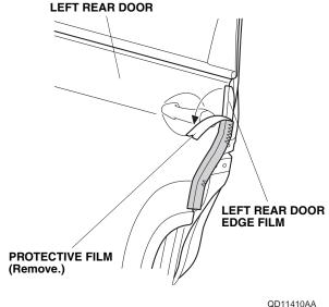
17. Starting from the center and working outward, use your finger to fold the left rear door edge film inside the left rear door. Move your finger in one direction only. Do not damage the door seam sealant.
