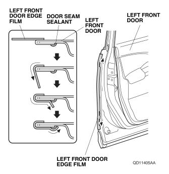
Using a shop towel, wipe the excess 3M protective tape application solution from the left front door edge film. Allow the left front door edge film to dry thoroughly.
