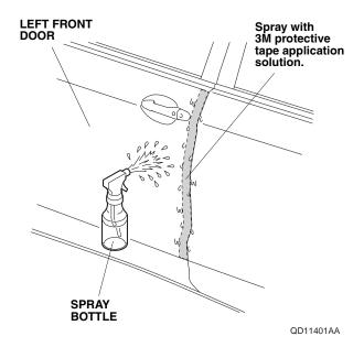
6. Open the left front door. Peel back about 50 mm (2.0 in.) of adhesive backing from the left front door edge film. Align the V-notch on the left front door edge film with the character line on the left front door.
