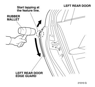
5. Repeat steps 3 through 14 to install the right door edge guards on the right side of the vehicle.
