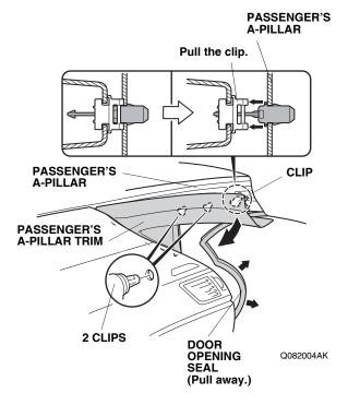
7. Pull out the passenger's A-pillar trim to release the clips.
