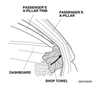
Remove the passenger's A-pillar trim from the upper clip (unplug the vehicle connector, if equipped). Carefully remove the shop towel and any clips that fell from the passenger's A-pillar trim. NOTE: The upper clip will stay in the body.
