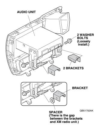
23. Install the XM radio unit to the brackets in the audio unit with four washer bolts.
