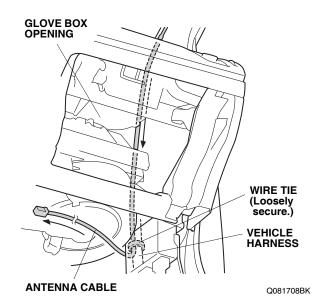
40. Route the antenna cable to the center panel opening as shown.
