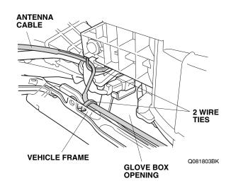
46. Cut one urethane tape, and wrap the piece of urethane tape around the antenna cable as shown.
