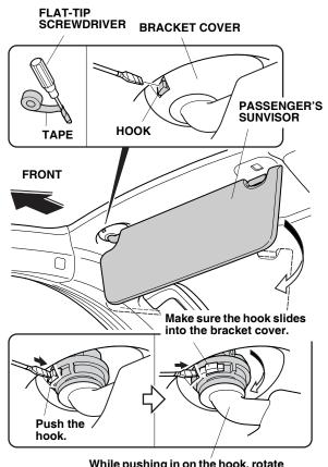
While pushing in on the hook, rotate the sunvisor backward about 45°.  $$_{\rm Q091503BK}$$
