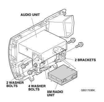
24. Secure two washer bolts installed in step 22.
