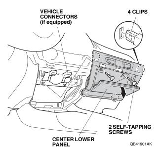
19. Remove two bolts and two self-tapping screws.
