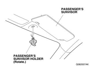
3. Wrap the end of a flat-tip screwdriver with tape. Locate the slot in the bracket cover, and insert a flattip screwdriver into the slot. Push the hook with the flat-tip screwdriver.
