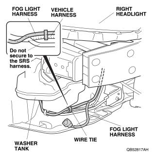
33. Locate the two vehicle clips. Secure the fog light harness to the vehicle harness with two wire ties as shown.
