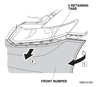
With the help of an assistant, remove the front bumper (two hex bolts and four clips). Place the front bumper on a blanket to prevent damage.
