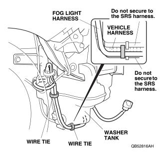
32. Under the washer tank, secure the fog light harness to the vehicle harness with one wire tie as shown. Do not secure the fog light harness to the SRS harness.
