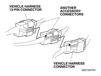
43. Remove the clip from the vehicle harness 13-pin connector, and install clip B on the vehicle harness 13-pin connector.
