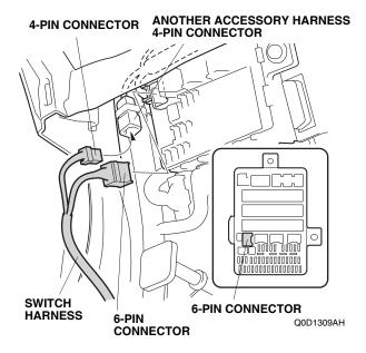
55. Secure the switch harness to the vehicle harness with two wire ties.
