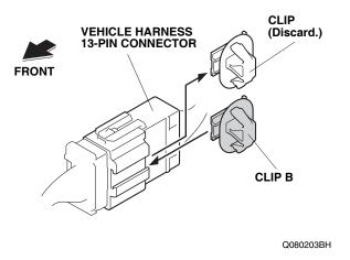
44. Unplug the vehicle harness 13-pin connector.
