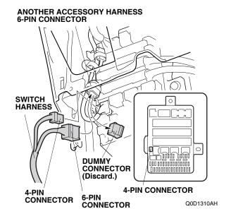
54. If the 4-pin connector is already used by another accessory, locate the 4-pin connector taped on another accessory harness. Plug the switch harness 4-pin connector into another accessory harness 4-pin connector.
