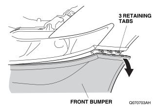
• On each side, release five retaining tabs.
