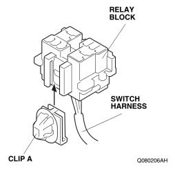
50. Install the relay to the switch harness relay block.
