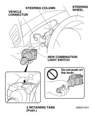
60. Plug the vehicle connector to the new combination light switch.
