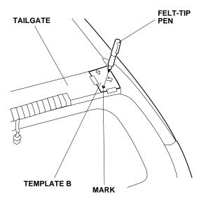
9. Remove the template. Turn the template over, and repeat steps 7 and 8 to mark the left side of the tailgate.
