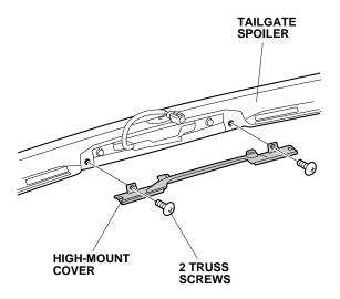
38. Bring the tailgate spoiler to the vehicle, and plug the tailgate spoiler 2-pin connector into the spoiler harness 2-pin connector.
