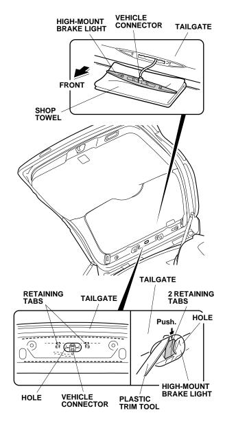
Gently close the tailgate. Unplug the vehicle connector, then remove the high-mount brake light. Remove the shop towel.
