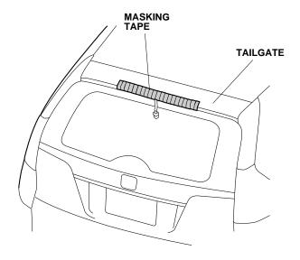
7. Place template B on the top right corner of the tailgate, and align it to the edge of the tailgate. Secure the template in place with masking tape.
