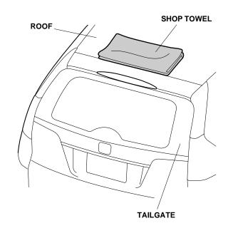
3. Open the tailgate. Remove the tailgate upper trim panel (four clips and two retaining tabs).
