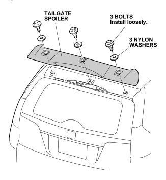
41. Use the palm of your hand to firmly press the tailgate spoiler to the tailgate. Make sure the hook and loop fasteners are secure.
