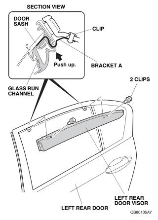
20. Secure the left rear door visor to two brackets A with two clips. Make sure to push up on the brackets A while installing two clips.
