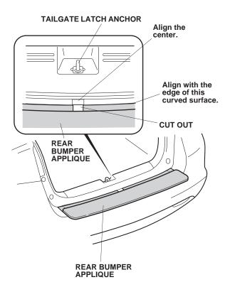
4. Remove the right adhesive backing from the rear bumper applique. Using the applicator with the soft sleeve, firmly press the forward section of the rear bumper applique against the bumper. Do not press the rear section at this time. If you see a bubble, stop and gently peel up that section to work out the bubble. Work slowly and keep pressure against the rear bumper applique.
