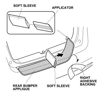
5. Remove the small right adhesive backing. Using the soft sleeve, firmly press the rear bumper applique against the rear bumper.
