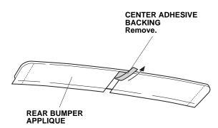
3. Place the rear bumper applique on the rear bumper, and align the cutout with the tailgate latch anchor. Be sure the rear bumper applique is aligned with the edge of the curved surface.
