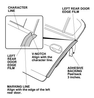
18. When the alignment is correct, apply light pressure to the door edge film while you carefully remove the adhesive backing. Don't worry about wrapping the door edge film around the door at this time.
