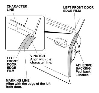
7. When the alignment is correct, apply light pressure to the door edge film while you carefully remove the adhesive backing. Don't worry about wrapping the door edge film around the door at this time. 8. Insert the applicator into the soft sleeve. Starting from the center and working outward, use the soft sleeve to smooth out the left front door edge film. Move the soft sleeve in only one direction.
