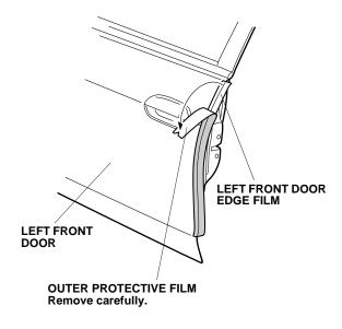
10. Starting from the center and working outward, fold the left front door edge film around the left front door edge. Be careful not to damage the door seal during this procedure.
