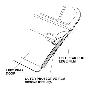
21. Starting from the center and working outward, fold the left rear door edge film around the left rear door edge. Be careful not to damage the door seal during this procedure.
