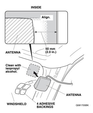
34. Remove four adhesive backings from the antenna, and attach the antenna in the location shown. Apply firm pressure to securely attach the antenna.
