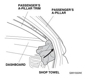
11. Remove the passenger's A-pillar trim from the upper clip (unplug the vehicle connector, if equipped).
