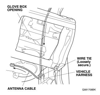
Route the antenna cable to the center panel opening as shown.
