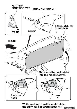
4. While pushing in on the hook, rotate the passenger's sunvisor backward about 45°. Make sure the hook slides into the bracket cover.
