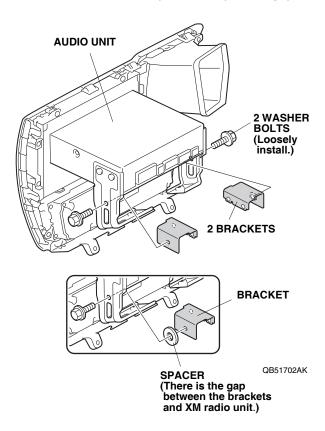
23. Install the XM radio unit to the brackets in the audio unit with four washer bolts.
