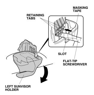
10. Use a flat-tip screwdriver wrapped with masking tape to release the three retaining tabs on the other side of the left sunvisor holder. Remove the holder.
