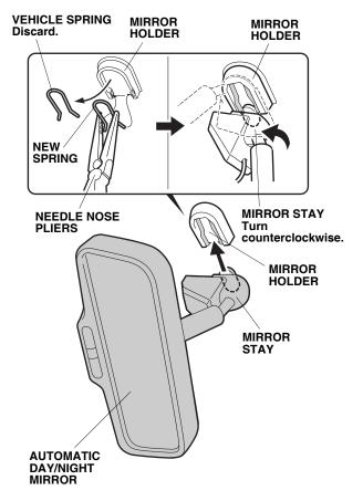
18. Slide the automatic day/night mirror stay into the mirror holder. Then turn the mirror stay counterclockwise to secure the automatic day/night mirror in the holder.
