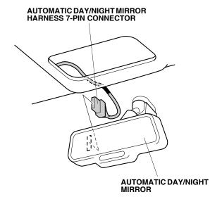
30. Align the green tape on the automatic day/night mirror harness with the edge of the headliner. Route the automatic day/night mirror harness through the grooves in the harness cover. Secure the harness cover to the mirror stay.
