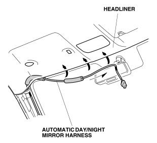
29. Plug the automatic day/night mirror harness 7-pin connector into the automatic day/night mirror.
