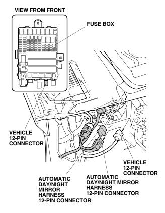
23. Secure the automatic day/night mirror harness to the vehicle harness with one wire tie.
