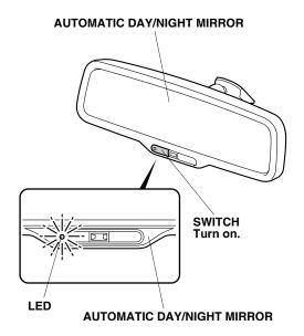
Cover the front sensor on the automatic day/night mirror with your hand, and use a flashlight to light the rear sensor on the mirror. Make sure the mirror surface dims.
