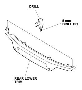
7. While wearing eye protection, drill the lower holes to 8 mm. First drill with a 5 mm drill bit, and finish with an 8 mm drill bit. Remove all burrs.
