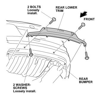
While applying light pressure against the rear lower trim, slowly and carefully remove the adhesive backings.
