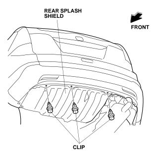
Position the rear lower trim on the rear bumper, and loosely secure the rear lower trim with three clips removed in step 1.
