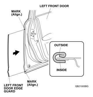
8. Starting at the feature line, use a rubber mallet to tap the left front door edge guard into position with a series of light taps, then work up and down. Make sure the position of the left front door edge guard is correct. Once in place, do not attempt to remove, reposition, or reinstall the left front door edge guard.
