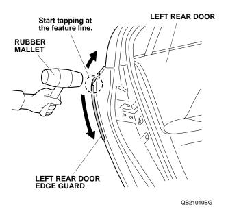
15. Repeat steps 3 through 14 to install the right door edge guards on the right side of the vehicle.
