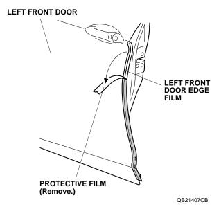
10. Starting from the center and working outward, use your finger to fold the left front door edge film inside the left front door. Move the your finger in one direction only. Do not damage the door seam sealant.
