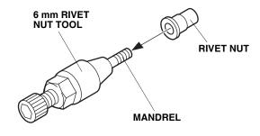
12. Insert the rivet nut into the hole in the trailer hitch, and insert the hex wrench in the 6 mm rivet nut tool.
