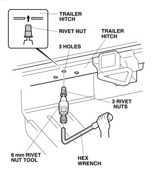
13. Holding the 6 mm rivet nut tool with the hex wrench, turn the 19 mm wrench clockwise and install the rivet nut to the trailer hitch.
