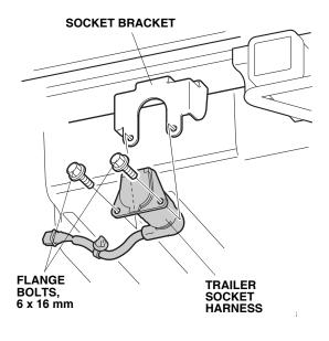
17. Plug the trailer socket harness 10-pin connector into the vehicle 10-pin connector.
