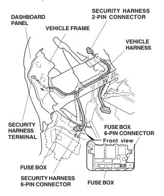
15. Route the security harness 2-pin connector along the vehicle harness. Route the security harness terminal between the vehicle frame and dashboard panel.
