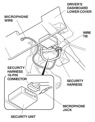
28. Fold the security harness and microphone wire, and secure them with one wire tie with no tension on the microphone jack.
