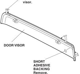
Push the two door visor brackets onto the door sash.
