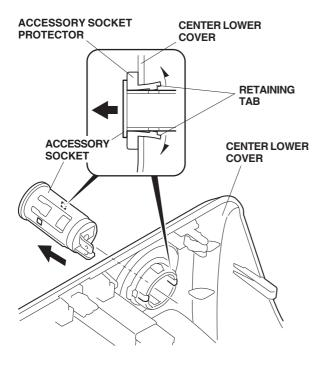
8. Remove the accessory socket protector from the dashboard center lower cover by releasing the two retaining tabs.
