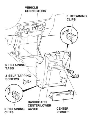
Insert a flat-tip screwdriver with a shop towel wrapped around it into the groove in the instrument panel, and release the clips. Pull the instrument panel out toward you to release the eighteen clips, and unplug the vehicle connectors. Remove the instrument panel.
