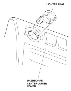
Align the locating tab from the socket with the cutout in the ring, and slide the cigarette lighter socket into the lighter ring. Push the cigarette lighter into the socket.
