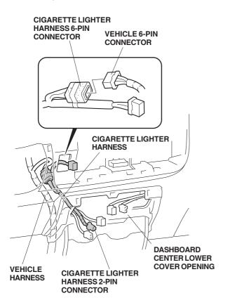
12. Connect the vehicle 2-pin connector and cigarette lighter harness 2-pin connector into the cigarette lighter socket. Reinstall the dashboard center lower cover.
