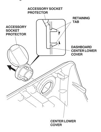
9. Slide the lighter ring into the hole in the front dashboard center lower cover in the direction shown.
