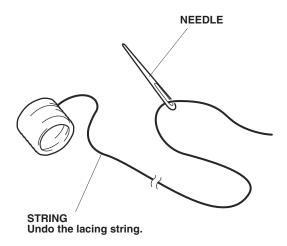
Starting at the back of the left spoke, lace the string through the holes of the steering wheel cover from the inside. Leave approx. 100 mm (3.93 in.) of string at the end. This will be used to tie the string when finished.
