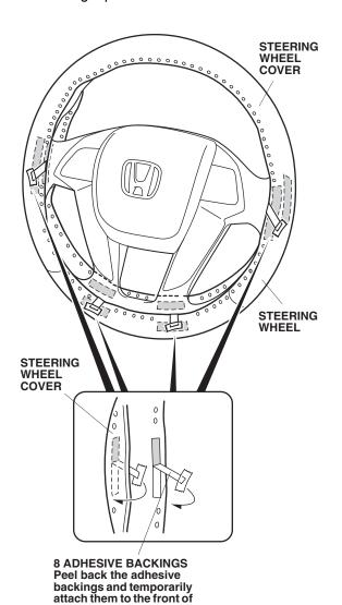
the steering wheel cover with masking tape.
