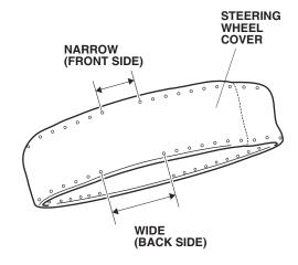
2. Place the wheel cover over the steering wheel with the unpierced sections of the wheel cover lined up with the spokes of the steering wheel as shown.
