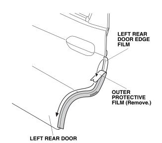
16. Starting in the middle of the door edge film and working outward, fold the film around the door edge using your fingers. Move your fingers in one direction. Attach the film over the seam sealant. Do not trim or damage the seam sealant.
