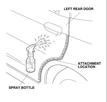
12. Open the left rear door again. Peel back about 50 mm (2 in.) of adhesive backing from the left rear door edge film. Align the V-notch in the door edge film with the end of the character line on the upper part of the left rear door.
