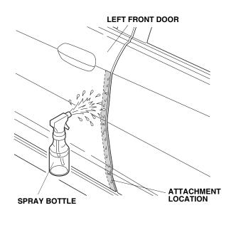
Open the left front door again. Peel back about 50 mm (2 in.) of adhesive backing from the left front door edge film. Align the V-notch in the door edge film with the end of the character line on the upper part of the front door.
