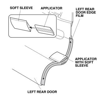
15. When you are satisfied that the door edge film is firmly attached to the door, slowly remove the outer protective film.
