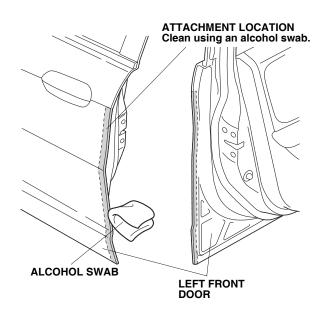
Close the left front door. Using a spray bottle with 3M protective tape application solution, spray the area where the left front door edge film will attach.
