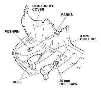
36. While wearing eye protection, drill each pierced mark on the rear under cover. First drill with a 3 mm drill bit, then enlarge each hole to 20 mm using a 20 mm hole saw.
