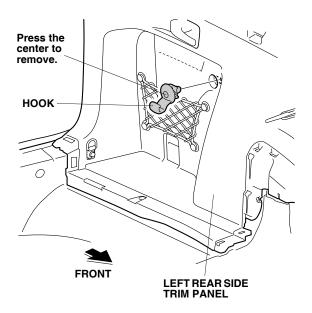
16. Remove the tie-down hook (one bolt).
