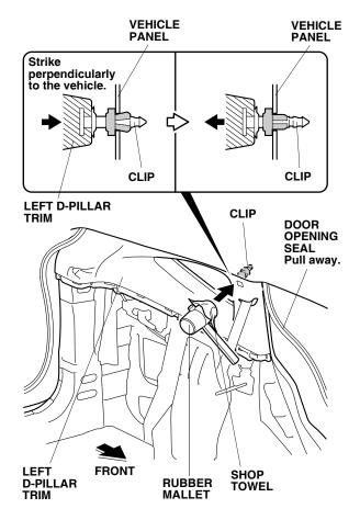
20. Using a rubber mallet wrapped with a shop towel, lightly tap the area marked "SIDE CURTAIN AIRBAG" on the left D-pillar trim to push in the clip. Make sure to strike area perpendicularly to the vehicle.
