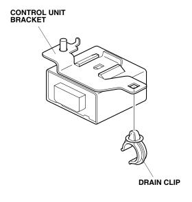
51. Install the control unit bracket to the vehicle panel with one 6 mm flange nut.
