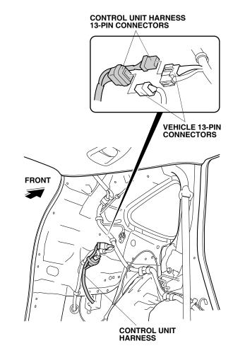
61. Route the control unit harness along the vehicle harness.
