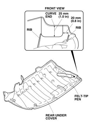
39. Using an air saw, cut the rear under cover at the mark made in step 38. Remove any burrs and sharp edges from the corners.
