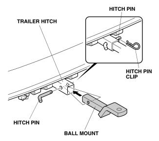
After the first 600 miles (1,000 km) of towing, have your Honda Dealer re-check the tightness of the trailer hitch bolts.
