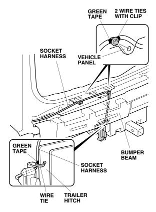
43. At the first green tape, secure the socket harness to the trailer hitch with one wire tie. At the next two green tapes, secure the socket harness to the vehicle panel with two wire ties with clip.
