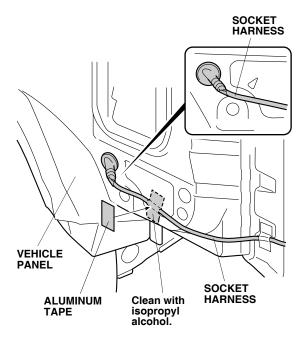
48. Inside the vehicle, secure the socket harness.
