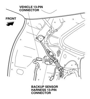
58. Plug the control unit harness 13-pin connector into the backup sensor harness 13-pin connector.
