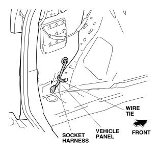
4WD vehicle: Route the socket harness along the vehicle harness and secure it to the vehicle harness with one wire tie.
