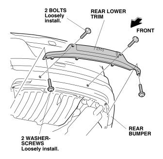
While applying light pressure against the rear lower trim, slowly and carefully remove the adhesive backings.
