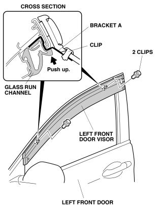
8. Adjust the end gap of the left front door visor as shown.
