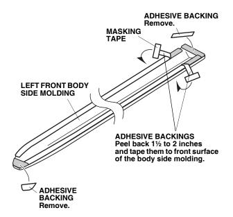
5. Align the end of the left front body side molding with the door edge as shown, and attach it along the top edge of the front template.
