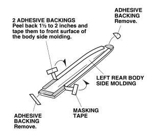
11. Align the end of the left rear body side molding with the body edge as shown, and attach it along the top edge of the rear template.
