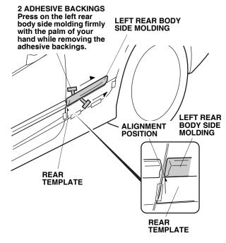
12. Press on the left rear body side molding firmly with the palm of your hand while removing the adhesive backings. Remove about 50 to 100 mm at a time.
