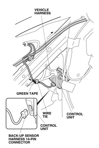
17. Secure the back-up sensor harness to the vehicle harness with two additional wire ties at the locations shown.
