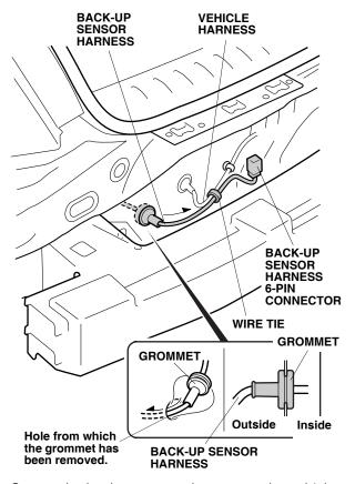
31. Secure the back-up sensor harness to the vehicle harness with one wire tie.
