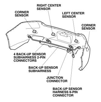
38. Attach the two center backup sensor subharness clips to the holes in each center sensor clip.
