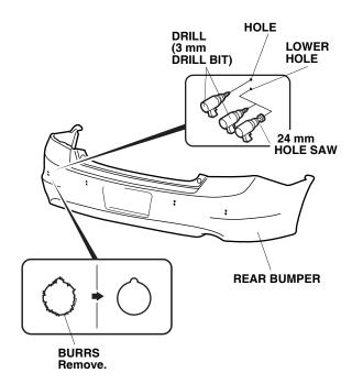
Using a 24 mm hole saw, enlarge the upper outboard hole on the right side of the bumper. Remove all burrs.
