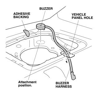
22. Remove the adhesive backing from the beeper, and attach it to the opening for the left rear speaker at the location shown. Route the beeper harness through the hole in the rear shelf.
