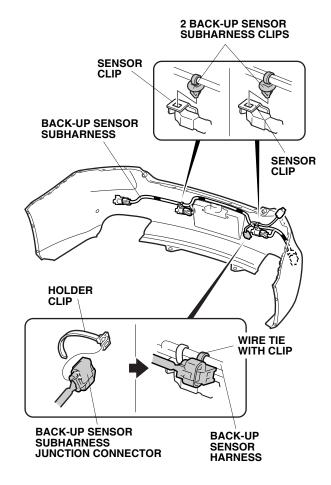
39. Attach one wire tie with holder clip to the back-up sensor subharness junction connector and secure the wire tie to the vehicle harness.
