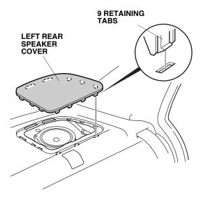
10. Remove the left rear speaker (one bolt and disconnect the vehicle connector).
