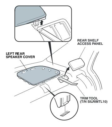
9. Remove the left rear speaker cover (nine retaining tabs).
