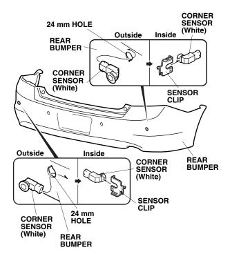
36. Install the two center sensors into the 26 mm holes in the rear bumper using the sensor clips. Note the direction and location for each sensor.
