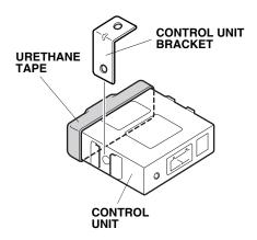
12. Install the control unit to the vehicle panel:
