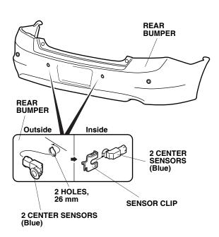
37. Plug the four back-up sensor subharness 2-pin connectors into the back-up sensor connectors.
