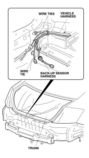
28. Install one wire tie with clip to the holder with the fuse case, and attach the wire tie to the vehicle harness.
