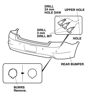
Using a 26 mm hole saw, enlarge both lower inboard bumper holes at the center of the bumper. Remove all burrs.
