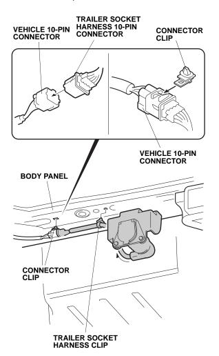
18. Install the connector clip into the vehicle 10-pin connector, and push the connector clip and trailer socket harness clip into the holes of the body panel.
