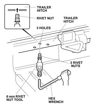
13. Holding the 6 mm rivet nut tool with the hex wrench, turn the 19 mm wrench counterclockwise and install the rivet nut to the trailer hitch.
