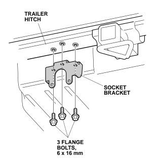
16. Install the trailer socket harness to the socket bracket with two 6 x 16 mm flange bolts.
