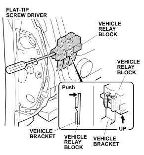
9. Attach the two relays into the vehicle relay block, and reinstall the vehicle relay block.
