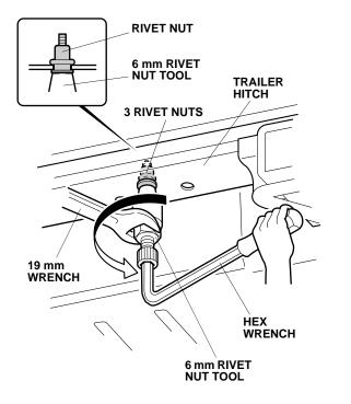
14. Remove the 6 mm rivet nut tool from the rivet nut by turning the hex wrench counterclockwise. Install two more rivet nuts in the holes in the trailer hitch.
