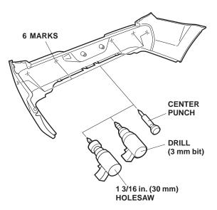
27. Measure 9 mm down from the top outside edge on the left side of the rear bumper, and mark the rear bumper with masking tape.
