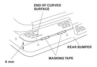
28. On the back of the left rear bumper trim, peel back 1 1/2 to 2 in. (3-5 cm) from each adhesive backing, and tape it to the front of the trim.
