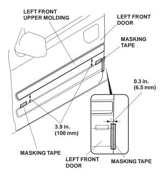
7. On the inside of the left front lower molding, attach a strip of masking tape to the ends of the long adhesive backing and peel back 1-1/2 to 2 in. (3-5 cm) of the adhesive backing. Tape the ends to the front of the moldings. Remove and discard all other adhesive backings.
