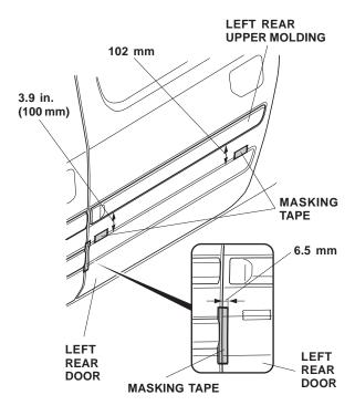
17. On the inside of the left rear lower molding, attach a strip of masking tape to the ends of the long adhesive backing and peel back 1-1/2 to 2 in. (3-5 cm) from the adhesive backing. Tape the ends to the front of the moldings. Remove and discard all other adhesive backings.
