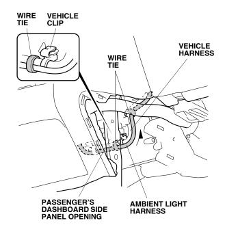
15. Route the ambient light harness along the vehicle harness, and to the blower motor. Secure the ambient light harness to the vehicle harness with two wire ties.
