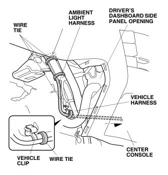
14. Route the ambient light harness along the vehicle harness, and secure it to the vehicle harness with two wire ties.
