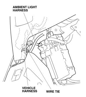
9. Install the ambient light to the hole in the dashboard as shown.
