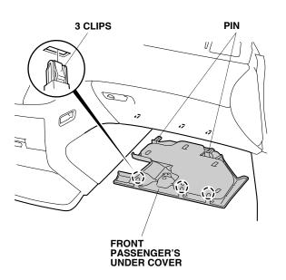
4. Remove the passenger's dashboard side panel (three clips, four retaining tabs, and one pin).
