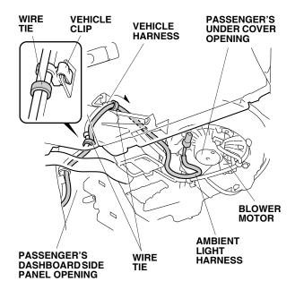
16. Secure the ambient light harness to the vehicle harness with three wire ties.
