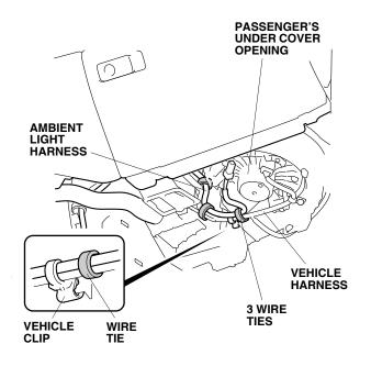
17. Install the ambient light to the passenger's under cover as shown.
