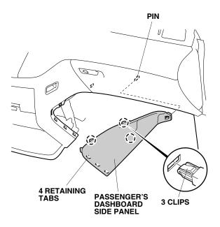
5. Remove the driver's dashboard side panel (three clips, four retaining tabs, and one pin).
