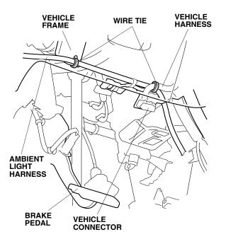
13. Route the ambient light harness through the center console, and secure it to the vehicle harness with three wire ties.
