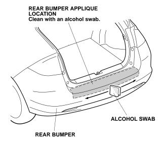
2. Remove the center adhesive backing from the rear bumper applique.
