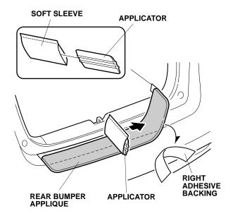
Remove the small right adhesive backing. Using the applicator, firmly press the rear bumper applique against the rear bumper.
