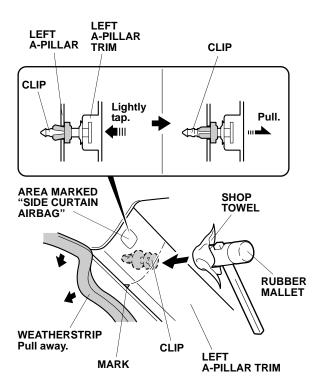
10. Using a rubber mallet wrapped with a shop towel, lightly tap the left A-pillar trim where it says "SIDE CURTAIN AIRBAG" to release the clip.
