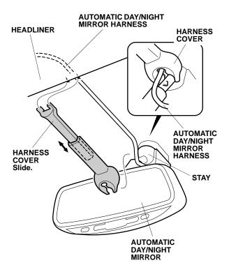
25. Secure the automatic day/night mirror harness to the headliner with one EPT sealer:
