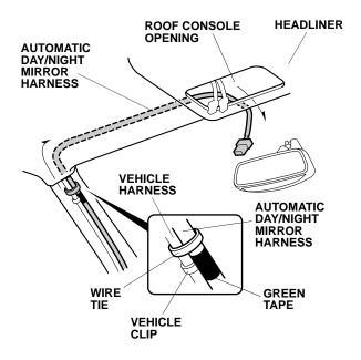
22. Secure the automatic day/night mirror harness to the vehicle harness with one wire tie at the green tape.
