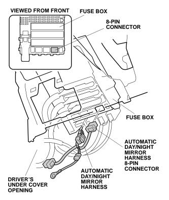
If the fog light connector is already plugged into the fuse box 8-pin connector, remove the dummy connector from the automatic day/night mirror harness.
