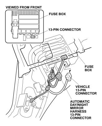
29. Plug the vehicle 13-pin connector into the automatic day/night mirror harness 13-pin connector.
