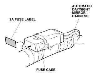
Using electrical tape, attach a piece of steel wire to the black connector on the automatic day/night mirror harness.
