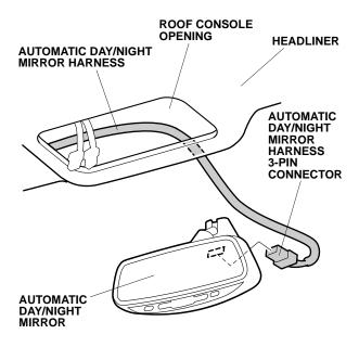
24. Route the automatic day/night mirror harness through the groove in the harness cover. Secure the harness cover to the stay, and slide the harness cover under the headliner.
