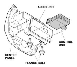
13. Plug the bus cable into the control unit and into the audio unit.
