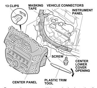
Remove the one screw. Using a plastic trim tool, pull the center panel out toward you to release the 13 clips. Unplug the vehicle connectors to remove the center panel. 10. Wrap one urethane tape around the USB cord in the area shown.
